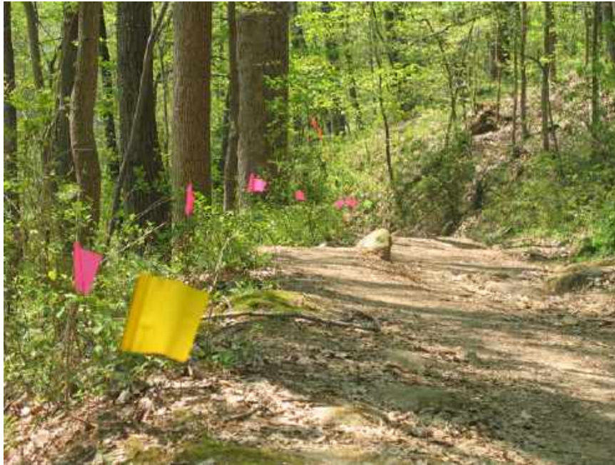
Figure 3-9. Track marked with several different colors of surveyor's flags. Yellow flags used for start, every 500 meters, and finish. Green flag marked with distance every 25 meters, red flags help clearly mark the track. Flagging tape used to initially layout the track.
