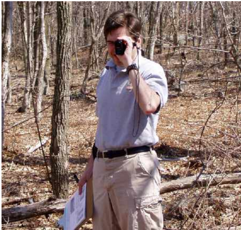
Figure 3-8. Hand-held Laser Range Finder in use.
